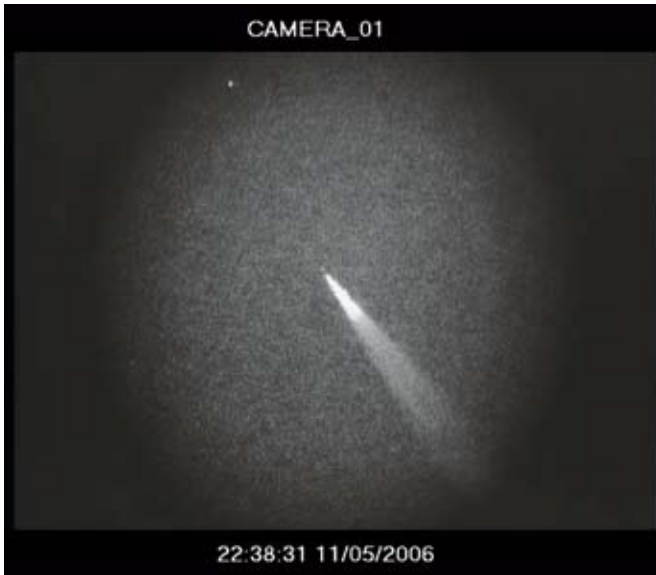
FIGURE 1 An image taken during laser ranging to GIOVE-A. Back-scattered laser light shows the path of the laser pulses through the atmosphere, and the faint sunlit image of GIOVE-A is visible at the tip of the "beam." A couple of stars are also visible in the field of view.
